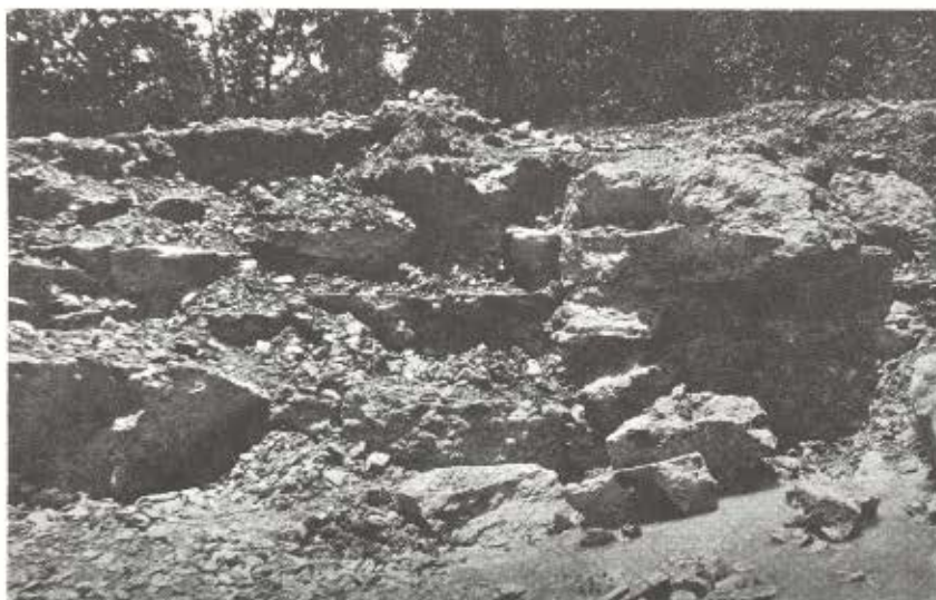
HARD ROCK-LIKE, finely porous high grade diaspore clay interbedded with thin seams of "mealy" clay at the Aufderheide pit in Gasconade County. Photo from McQueen, 1943.
