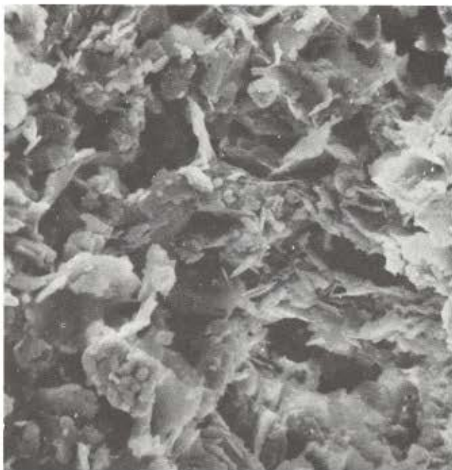
FIRST-GRADE DIASPOIRE CLAY 70% Al_2O_3 , 3,000X; Forbes Pit, Rolla, Mo. (2759)
