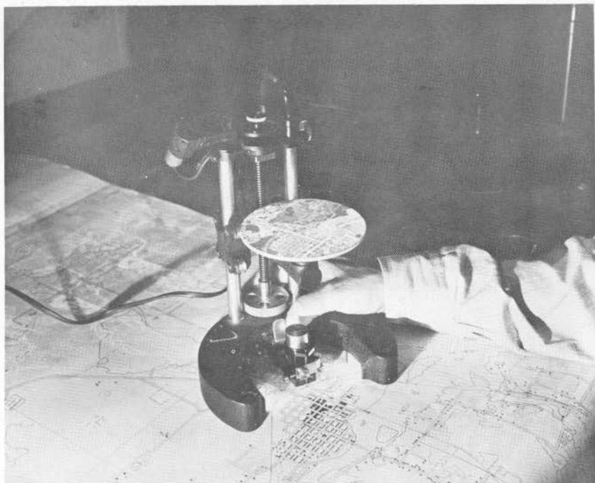
Fig. 10. Multiplex tracing table. A Bausch and Lomb multiplex tracing table showing how detail from the stereoscopic image is projected onto the mapping surface. The entire table is mounted on roller bearings and can be moved to any desired position on the map by the operator.
