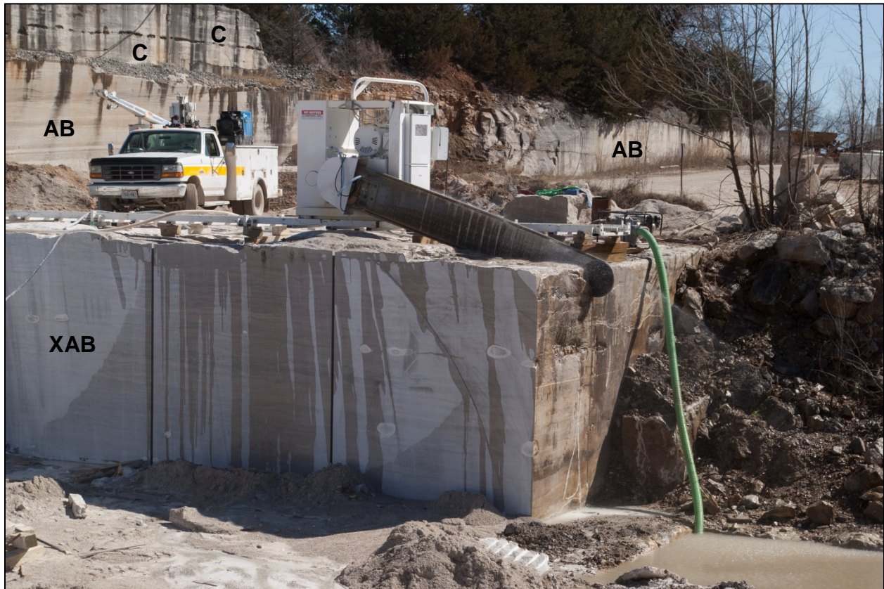
Figure 10. Present-day Phenix Marble Co. cutting out a block from quarrymen's ledge "XAB" on March 2, 2017. Ledges "C" and "AB" are visible in background. "AB" ledge in background was cut with a long wire saw by Carthage Marble Co. during the 1960s. View is facing south. (D.L. Bridges photograph)
