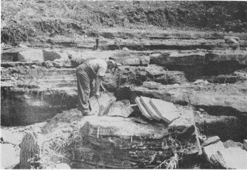
A. Sandstone slabs for small home construction being quarried in O. F. Beushausen quarry north of Ava, Douglas County, Missouri.
