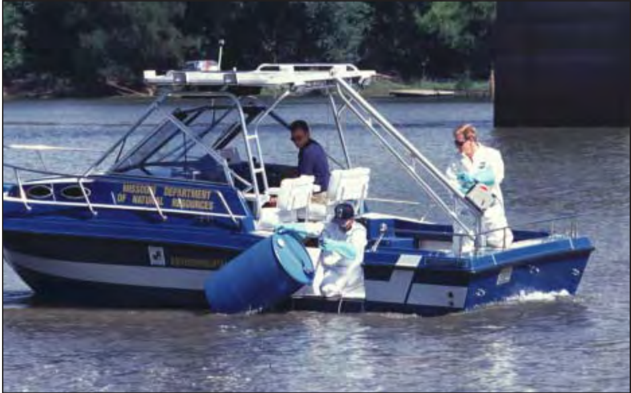
The department's environmental emergency response boat equipped for responding to petroleum and other chemical spills on major waterways. Photo from Environmental Service Program.
