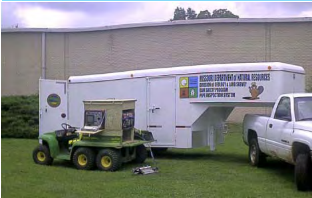
Tractor mounted pipe inspection camera system. Source: Dam and Reservoir Safety Program.
