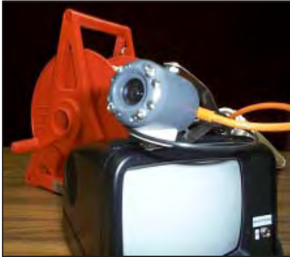
Downhole video camera. Camera head is less than 2 inches in diameter. Photo by Bruce Netzler.
