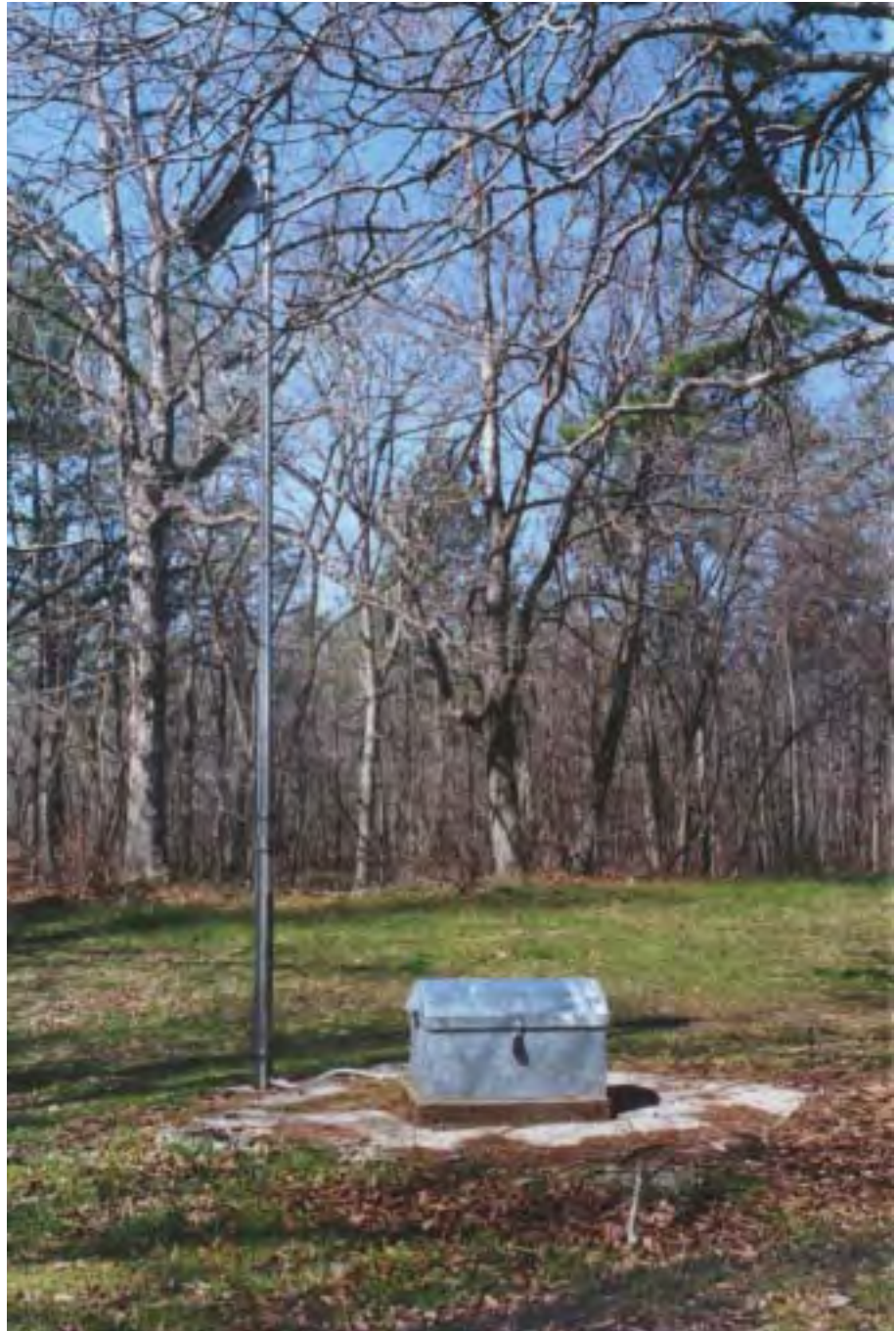
Wave of the future – new observation well recorders. These new data collection platforms consist of electronic data recorders and digital encoders. Water level information from each observation well is transmitted via satellite every four hours, allowing almost instantaneous access to important data. Photo by Susan Dunn.
