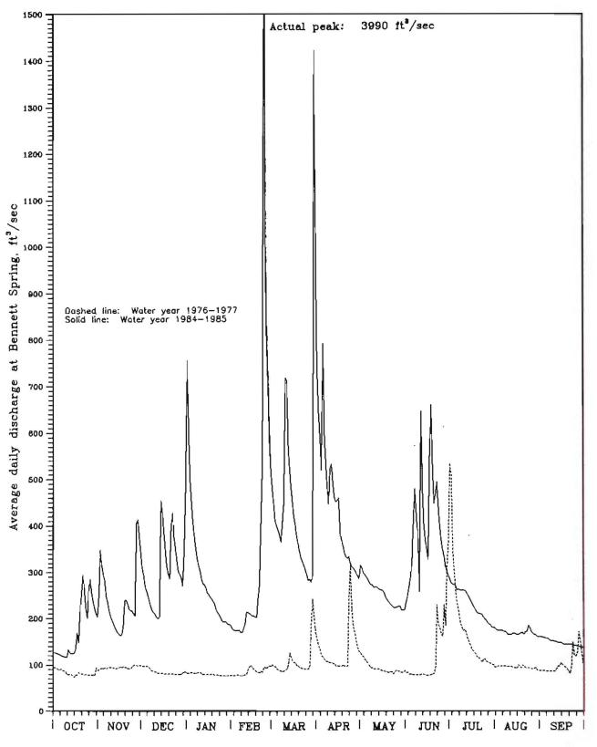
Figure 41: Hydrographs showing average daily flows at Bennett Spring during extremely wet and extremely dry years. Data source: U.S. Geological Survey.
