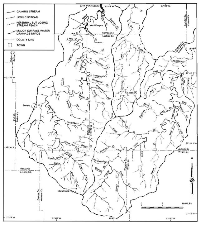
Figure 3: Galning and losing streams in the Bennett Spring study area.
