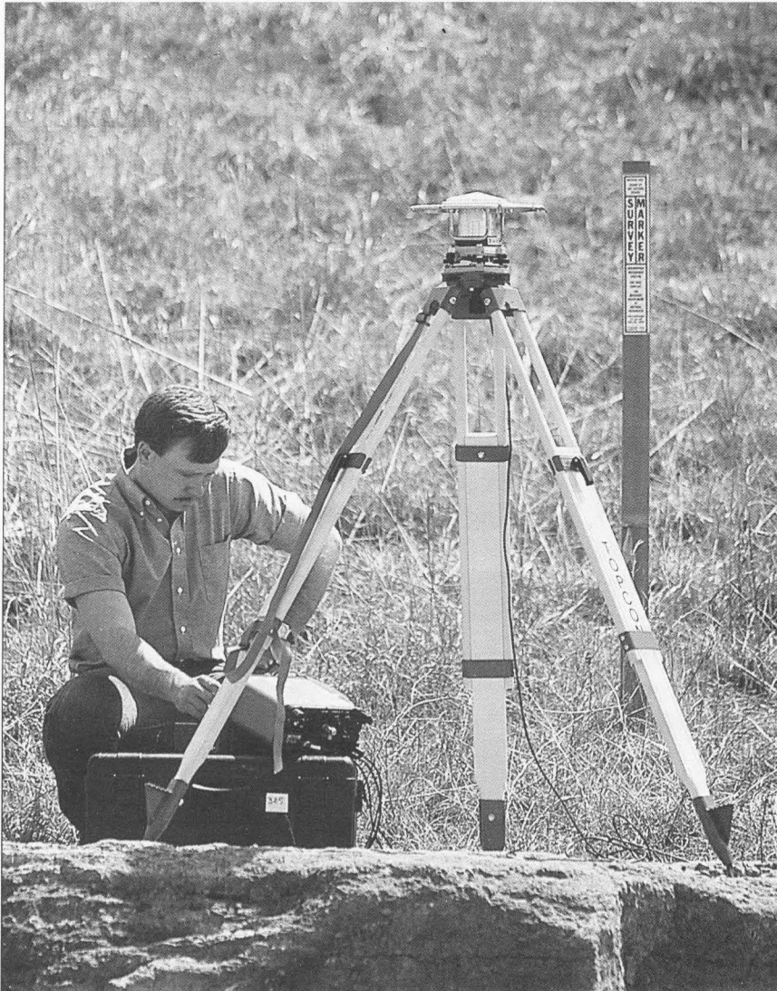
A land surveyor uses the Global Positioning Satellite System, which employs satellites to determine the equipment's position.
