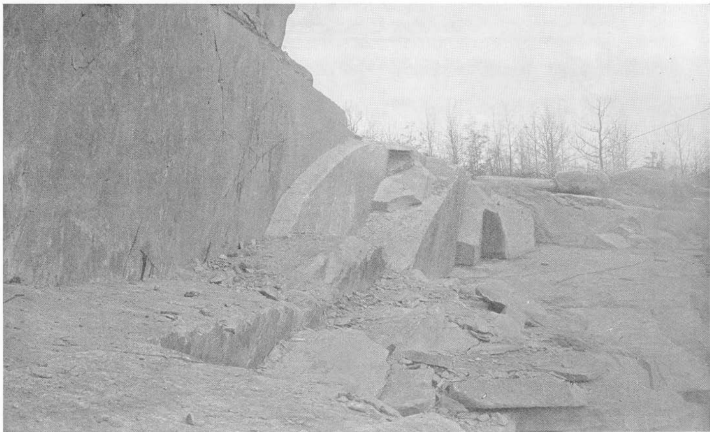
JOINTING OF GRANITE QUARRY OF SYENITE GRANITE CO., GRANITEVILLE.
